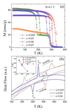
FIG. 2. (a) Temperature dependence of the magnetization [M(T)] measured during heating and cooling under the application of 0.1 T magnetic field. (b) DSC heat flow curves as a function of temperature measured at a rate of 20 K/min. The maxima and minima indicate the endothermic and exothermic behaviors during heating and cooling cycles, respectively. Inset: The transition temperatures as a function of Zn concentration.
