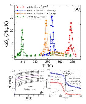
FIG. 3. (a) Plot of the magnetic entropy changes  $(-\Delta S_M)$  as a function of temperature for different magnetic field changes of  $\Delta H = 5$  (solid symbols) and 2T (open symbols), respectively. (b) The isothermal magnetization measured during heating in the vicinity of  $T_M$  for  $x\,{=}\,0.05$ . (c) Heating thermomagnetization curves for applied fields H = 0.1 and 5 T, respectively, to estimate the value of  $-\Delta S_M$  for x = 0.05 using Clausius-Clapeyron equation.
