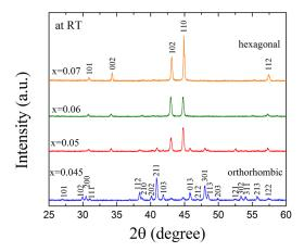
FIG. 1. XRD patterns of MnCo<sub>1-x</sub>Zn<sub>x</sub>Ge measured at room temperature.
