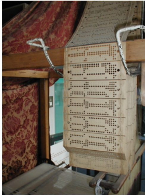
Figure 2. Jacquard Punch-Card Operated Loom (Image courtesy of Wikipedia).
