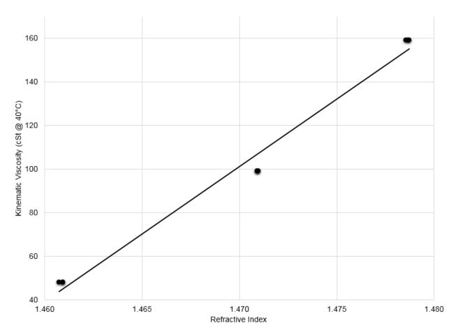
**Fig. 5** Actual refractive indices (round markers) (n=9) and predicted kinematic viscosity at  $40^{\circ}$ C (trend line) based on linear regression of refractive indices at 1.25 THz ( $R^2 = 0.9827$ , RMSE = 6.63)
