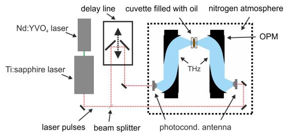
Fig. 1 Schematic of the THz time-domain spectrometer
