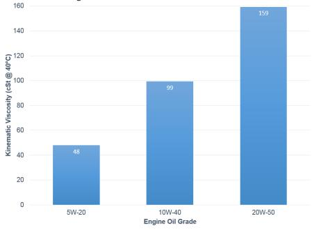
Fig. 2 Kinematic viscosity (cSt @ 40°C) for each engine oil grade based on ASTM D445
