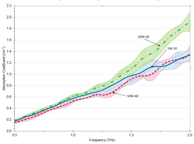
**Fig. 4** Mean absorption coefficient (n=3) of three fresh oil samples of different grades with 95% confidence interval bars
