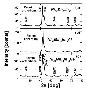
FIG. 1. Room temperature XRD patterns of  $Ni_{50}Mn_{35}In_{15},\,Ni_{50}Mn_{35}In_{14}Al,$  and  $Ni_{50}Mn_{35}In_{14}Ge.$
