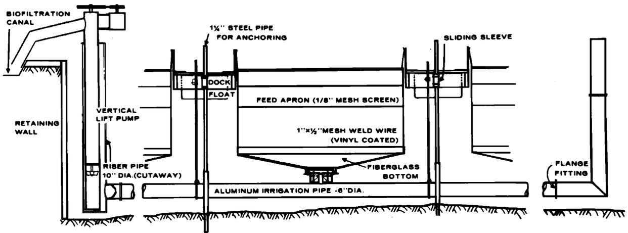
Fig. 1. Schematic drawing of a fish-rearing system that incorporates mechanisms for removing solid waste from cages.
