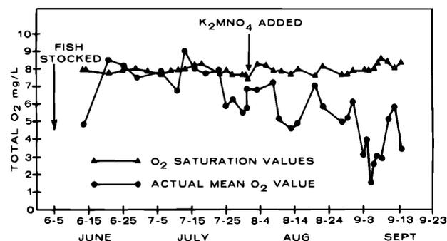
Fig. 3. Dissolved oxygen in a pond supporting a rearing system for caged fish. Readings were taken between 0900 and 1100 h in 1973.
