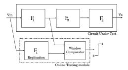
Figure 1. Redundancy based On-line testing.
