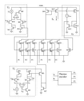
Figure 5. Proposed adaptive biasing circuit.
