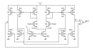
Figure 3. Proposed comparator sub-circuit.
