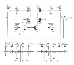
Figure 4. Modified comparator sub-circuit.
