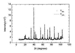
FIG. 1. Neutron diffraction pattern measured at 20 K for  $LaNi_{3,5}Mn_{1,5}$  and a fit based on the CaCu<sub>5</sub>-type structure and the ferrimagnetic mode.
