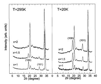
FIG. 2. Neutron diffraction patterns at 295 and 20 K for the  $LaNi_{5-x}Mn_x$  samples. All peaks are normalized to the 111 reflections, which are not shown in the patterns.
