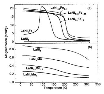
FIG. 3. Magnetization vs temperature for (a)  $\text{LaNi}_{3-x}\text{Fe}_x(H=1000 \text{ Oe})$  and (b)  $\text{LaNi}_{5-x}\text{Mn}_x(H=2000 \text{ Oe})$ .
