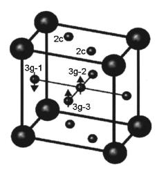
FIG. 4. LaNi<sub>5-x</sub>Mn<sub>x</sub> structure showing the antiparallel coupling of the manganese 3g moments. The larger atoms are La and the smaller ones are either Ni or Mn.
