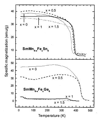
FIG. 1. Temperature dependence of the magnetization for  $SmMn_{6-x}Fe_xGe_6$  and  $SmMn_{6-x}Fe_xSn_6$  measured at an applied field of 0.2 T.
