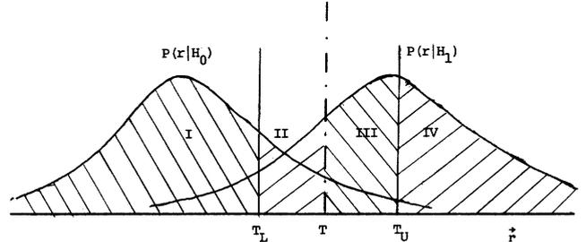
Fig. 5. Data distribution at each sensor under hypotheses  $H_1$  and  $H_0$ , and confidence regions. Threshold is indicated by  $T$ . The intervals  $(-\infty, T_L)$  and  $(T_U, \infty)$  are designated "confidence" regions. Interval  $(T_L, T_U)$  is designated "no confidence" region.
