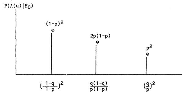
Fig. 1. Distribution of LR at fusion center under hypothesis  $H_0$  for two similar sensor system,  $N = 2$
