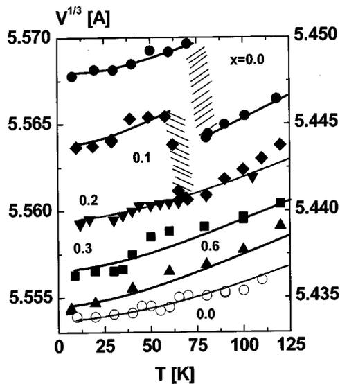
FIG. 4. Temperature dependence of the unit cell parameter  $V^{1/3}=(a^2c)^{1/3}$  for some characteristic samples of  $Tb_{1-x}Y_xMn_2Ge_2$  (full symbols, left scale) and  $TbMn_2Si_2$  (open symbols, right scale). The hatched regions show the area of coexistence of the phases in two Ge-containing compounds with a volume expansion at  $T_C^{(Tb)}$ .
