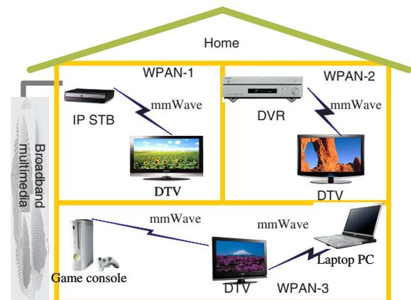
Fig. 1. Configuration of Gigabit WPANs.
