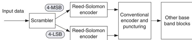
Fig. 3. Block diagram of the PHY layer (transmitter) in the UVoW.
