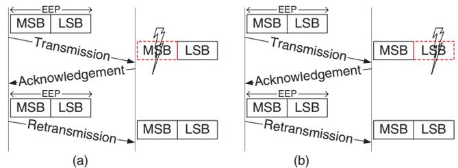
Fig. 5. Traditional ARQ schemes use single CRC. Even partial bits are received correctly; the sender retransmits another copy of the original packet.
