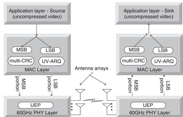
Fig. 2. UVoW system architecture.
