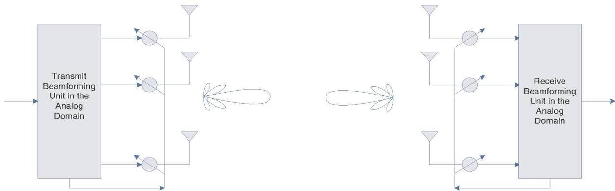
Fig. 1. Illustration of the antenna array beamforming.
