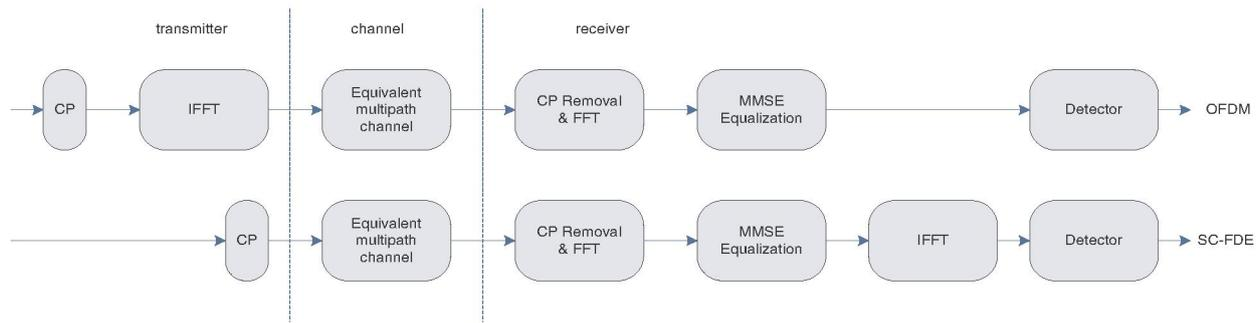
Fig. 2. System Diagrams of OFDM and SC-FDE.
