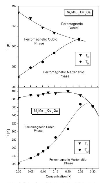
FIG. 1. (*T*-*x*)-phase diagram for  $Ni_2Mn_{1-x}Cu_xGa$  and  $Ni_2Mn_{1-x}Co_xGa$ .
