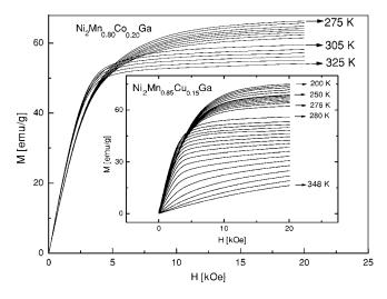
FIG. 2. The typical results of isothermal magnetization measurements M(H) for the Ni<sub>2</sub>Mn<sub>0.89</sub>Co<sub>0.20</sub>Ga. Inset: M(H) for the Ni<sub>2</sub>Mn<sub>0.85</sub>Cu<sub>0.15</sub>Ga.
