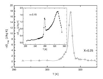
FIG. 4. Ni<sub>2</sub>Mn<sub>1-x</sub>Cu<sub>x</sub>Ga magnetic entropy change for  $\Delta H$ =+20 kOe and compounds with x=0.15 and 0.25.
