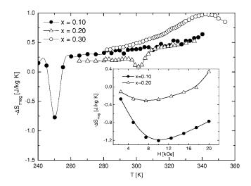
FIG. 3. Ni<sub>2</sub>Mn<sub>1-x</sub>Co<sub>x</sub>Ga magnetic entropy change for  $\Delta H$ =+20 kOe and compounds with x=0.10, 0.20, and 0.30. Inset: field dependence of  $\Delta S_{mag}$  at T= $T_M$ .
