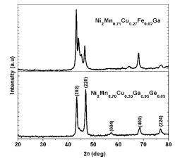
FIG. 1. Room temperature powder XRD patterns of  $Ni_2Mn_{0.71}Cu_{0.27}Fe_{0.02}Ga$  and  $Ni_2Mn_{0.70}Cu_{0.30}Ga_{0.95}Ge_{0.05}$ .
