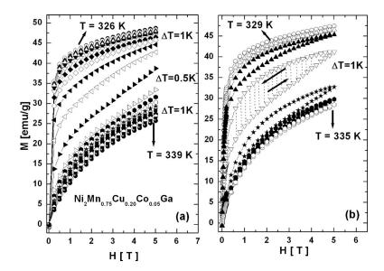
FIG. 4. (a) Isothermal magnetization curves of  $Ni_2Mn_{0.75}Cu_{0.20}Co_{0.05}Ga$  at temperature increments of 1 and 0.5 K and (b) the hysteresis loops of  $Ni_2Mn_{0.75}Cu_{0.20}Co_{0.05}Ga$  at temperatures where the maximum entropy is observed.
