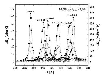
FIG. 5. Magnetic entropy changes  $(\Delta S_m)$  as a function of temperature of Ni<sub>2</sub>Mn<sub>0.75</sub>Cu<sub>.25-x</sub>Co<sub>x</sub>Ga for a field change ( $\Delta H$ ) of 5 T (closed symbols) and 2 T (open symbols).
