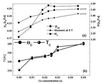
FIG. 3. (a) Magnetic moment ( $\mu_B/f.u.$ ) at 5 T, estimated saturation magnetic moment, and effective paramagnetic moment ( $p_{eff}$ ) and (b) paramagnetic Curie temperature,  $\Theta_C$ , and the Curie temperature,  $T_C$ , as a function of Co concentration of Ni<sub>2</sub>Mn<sub>0.75</sub>Cu<sub>0.25-x</sub>Co<sub>x</sub>Ga.
