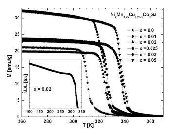
FIG. 2. Magnetization as a function of increasing temperature of  $Ni_2Mn_{0.75}Cu_{.25-x}Co_xGa$ , obtained at a field of 1 kOe. The inset shows the thermal expansion as a function of temperature for the alloy with x=0.02.
