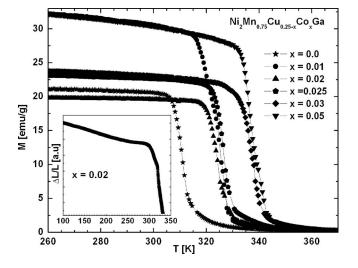
FIG. 2. Magnetization as a function of increasing temperature of  $Ni_2Mn_{0.75}Cu_{.25-x}Co_xGa$ , obtained at a field of 1 kOe. The inset shows the thermal expansion as a function of temperature for the alloy with x=0.02.
