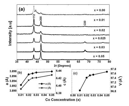
(a) Powder XRD patterns Ni<sub>2</sub>Mn<sub>0.75</sub>Cu<sub>0.25-x</sub>Co<sub>x</sub>Ga, (b) lattice parameters as a function of Co concentration, and (c) cell volumes as a function of Co concentration.
