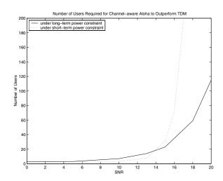
Fig. 3. Number of users required for Channel-aware ALOHA to outperform TDM under both short-term and long-term power constraints.
