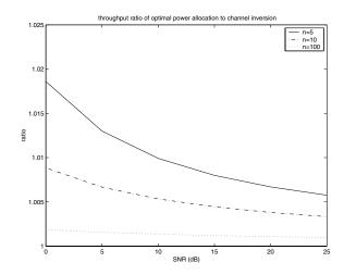
Fig. 1. Ratio of the throughput with optimal power allocation to that with channel inversion versus the expected received SNR for n=5,10,100 users.
