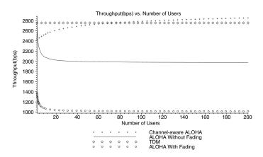
Fig. 2. Comparison of throughput versus the number of users under a short-term power constraint. The parameter used here are  $W=1 {\rm KHz}, P_m=40 {\rm W},$   $N_0=0.001$  and  $h_0=1$ .
