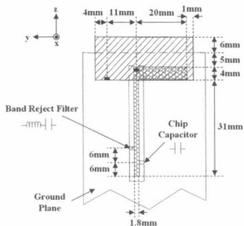
Figure 5. Dimension of the proposed antenna (top view)
