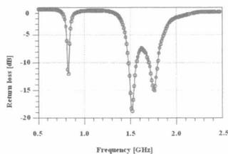
Figure 6. Measured return loss of the combined circuit
