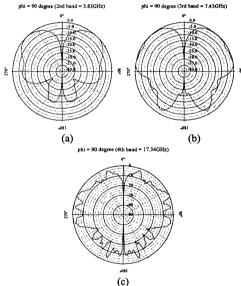
Figure 3. Radiation pattern of the modified truncated triangle gasket monopole antenna with  $\phi=90^\circ$ . (a)  $2^{nd}$  band = 3.83GHz, (b)  $3^{nd}$  band = 7.43GHz, and (c)  $4^{th}$  band = 17.34GHz.
