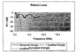
Figure 2. Return losses of the three Sierpinski monopole antennas.
