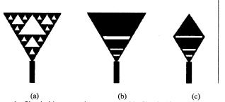
Figure 1. Sierpinski monopole antennas. (a) Sierpinski triangle gasket, (b) modified triangle gasket, and (c) truncated version of modified triangle gasket.
