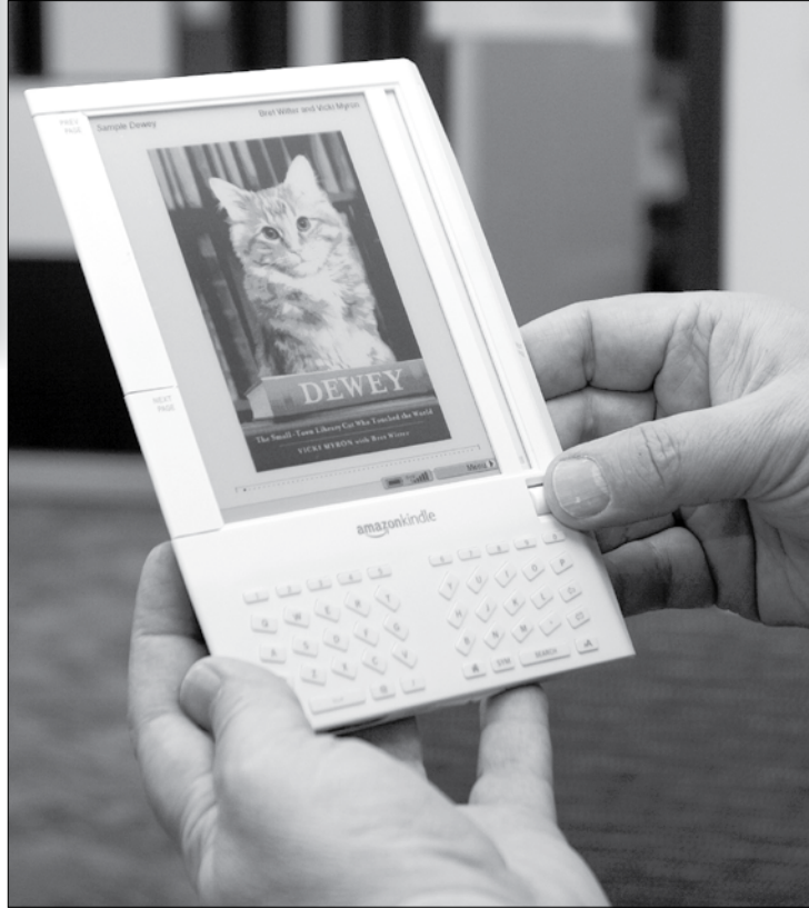
The Kindle has a six-inch diagonal screen that uses “electronic ink” that looks like ink on paper, not backlit like a computer or cell phone screen.
