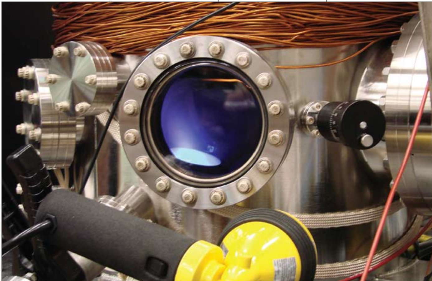
This instrument, a reactive unbalanced magnetron sputtering machine, uses high voltage to create a plasma that deposits a so-called “chameleon” coating on a substrate. The coatings change the characteristics of their surface or “skin” depending on the environment, lowering friction or boosting hardness as needed. Photo by Tim Crosby.
