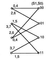
Fig. 3. 4-state 8-PSK Trellis Diagram.
