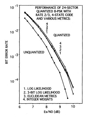
Fig. 8. Bit error rate performance for various metrics.
