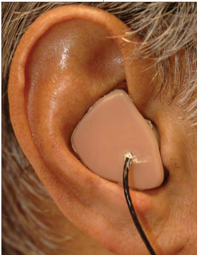
Lalit Gupta demonstrates a device that measures air pressure changes in the Eustachian tube caused by moving one's tongue. A company called Think-a-Move recently began marketing a wheelchair based on the technology.
