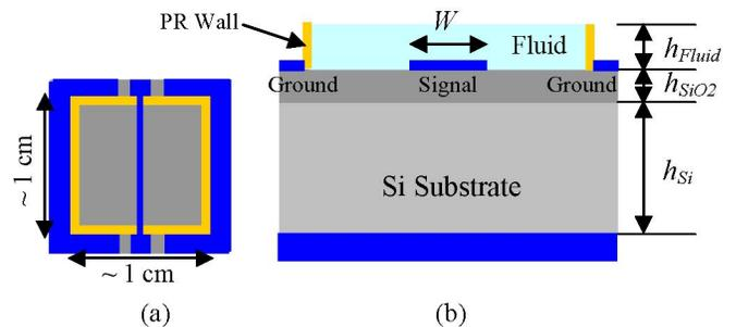
Fig. 1. Schematic of an on-chip microstrip transmission line. (a) Top view. (b) Cross-section view. Drawing not to scale.
