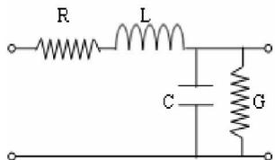
Fig. 2. A generic equivalent circuit model of on-chip transmission line.
