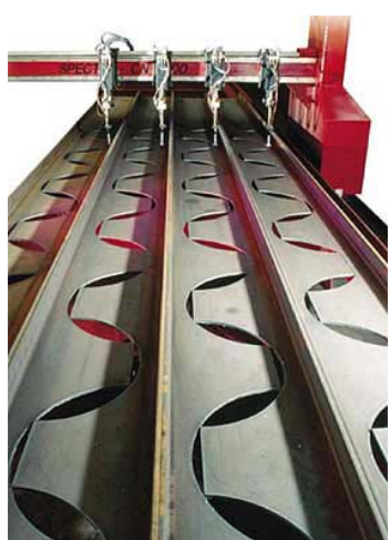
Figure 4.4. Manufacturing Process of Cellular Beams. Source: westok.co.uk.
