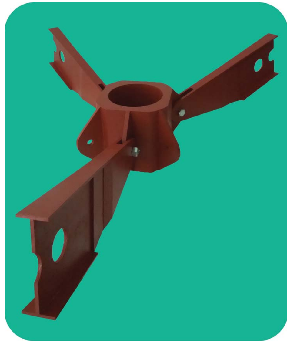
Figure 6.7c Fabricated half scale model of column sleeve connection. Source: Author
