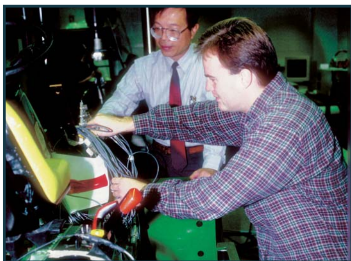
▲ Going nowhere fast: Accelerated lifespan testing of prototype lawn tractors made of composite materials has been funded by the John Deere Foundation and NSF.
