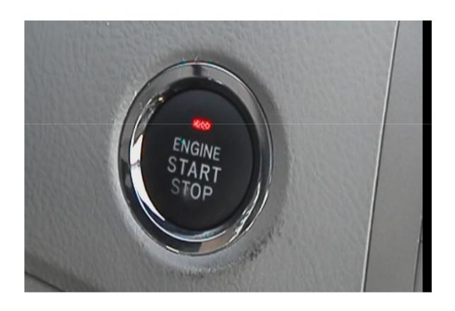
(continued): If brake switch operation is good check the 12 volt start signal to the PCM on the Acura and Toyota. The Dodge is more reliant on CAN.
