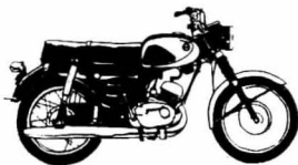
Suzuki Olympian 150 cc Touring Cycle 16 hp, twin-cylinder, 4-speeds, electric and step starter.
