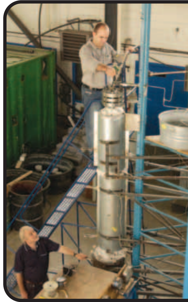
▲ Tomasz Wiltowski (left) looks on as graduate student Lubor Stonawski makes adjustments to a pilot-scale experimental gasification system that can separate carbon dioxide from hydrogen.
