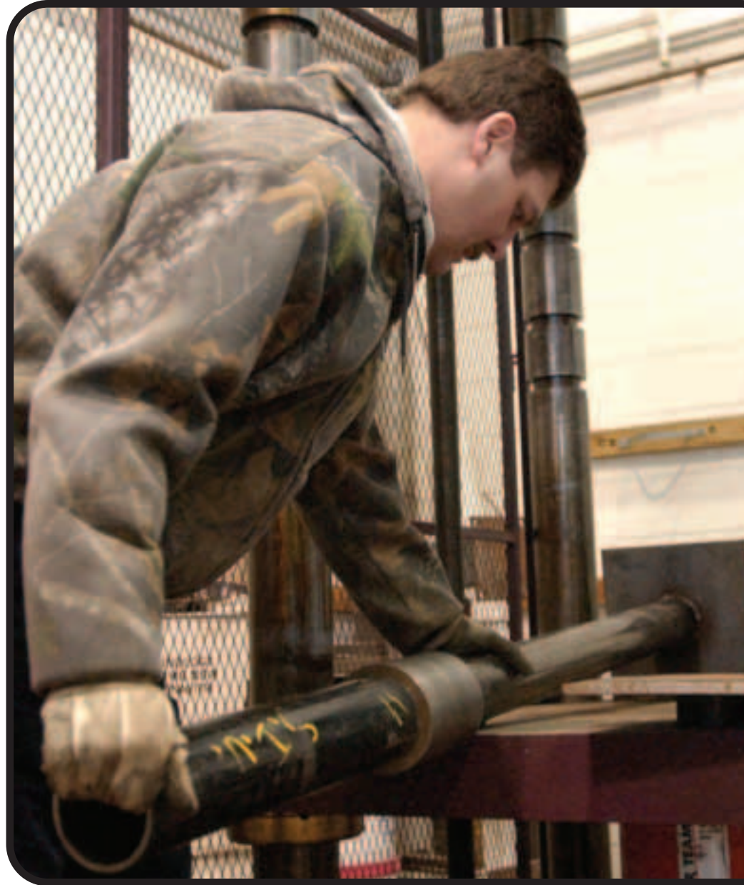
▲ Using a hydraulic lift, Bane Kroeger tests the new type of mine roof prop he designed.
