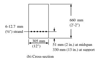
Figure 3. Pretensioned beam with single-point depressed strands for Example 2
