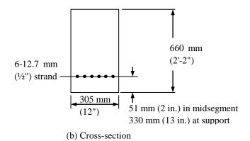
Figure 4. Pretensioned beam with two-point depressed strands for Example 3
