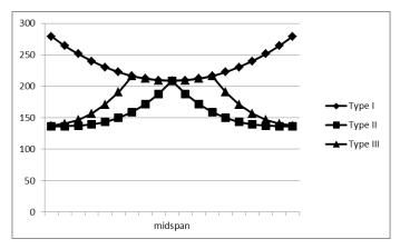
Figure 5. Prestress loss distributions along the beams in Examples 1, 2, and 3
