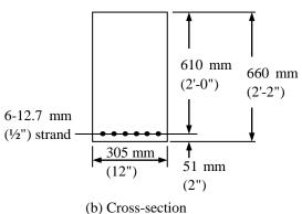
Figure 2. Pretensioned beam with straight strands for Example 1
