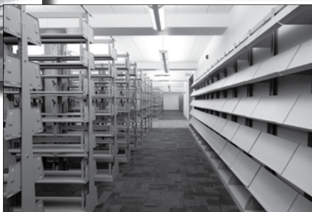
Miles of shelving will accommodate the millions of books home to Morris Library. An additional support bar along the third shelf makes this shelving seismically assured.
