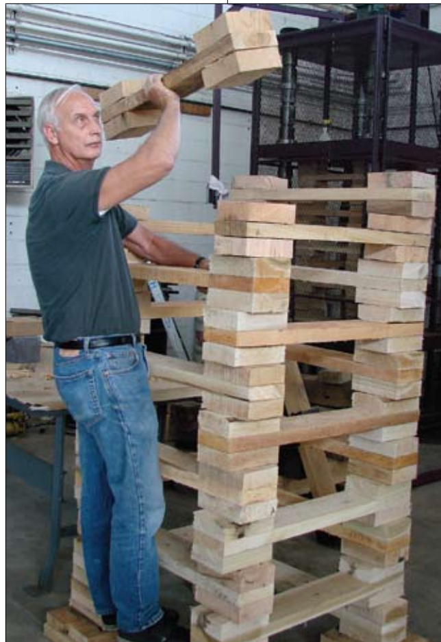
John Pulliam, researcher in mining and mineral resources engineering, demonstrates the ease with which miners can handle a new cribbing support system designed by Yoginder Paul Chugh and colleagues.
