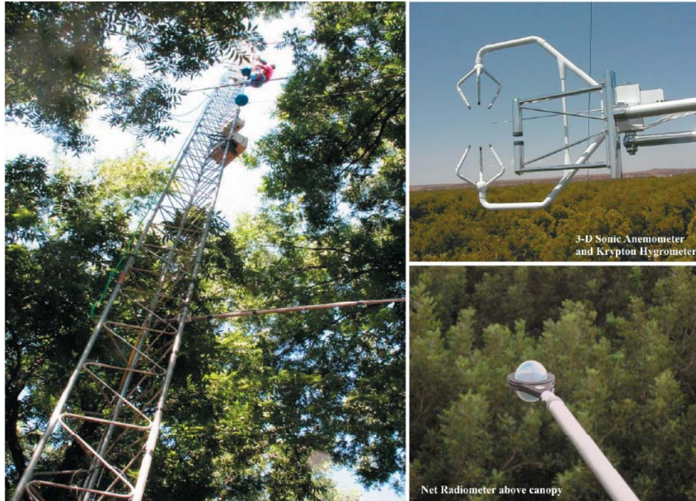
Figure 1. Eddy covariance flux tower installed in pecan orchard in Mesilla Valley, New Mexico.
