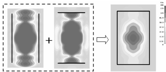
Fig. 3. Electric field distribution in the near field with the vertical reflector.
