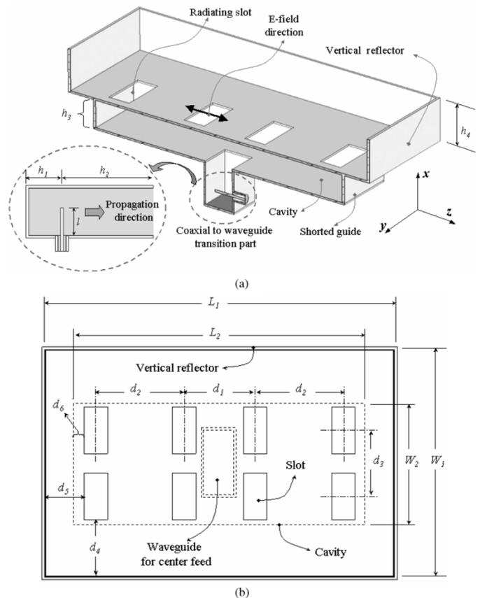
Fig. 1. Structure of the proposed antenna. (a) Three-dimensional cross sectional view. (b) Top view.
