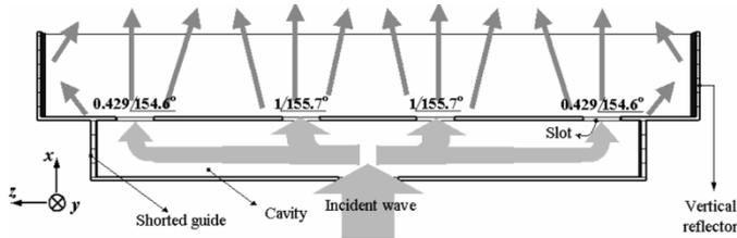
Fig. 2. Approximated field distribution within CBSAA by Ansoft's HFSS software.
