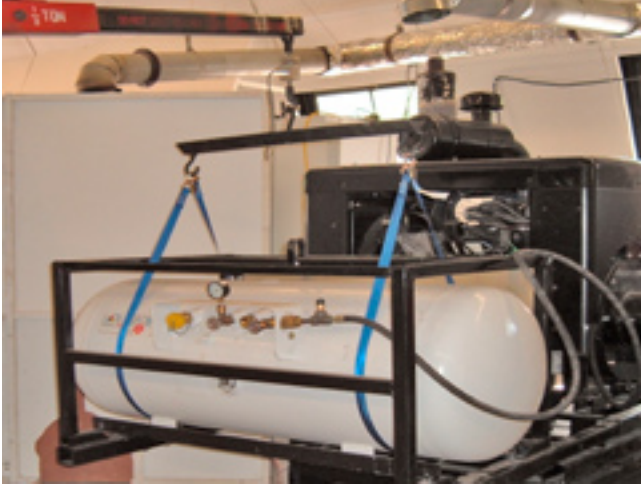
FIGURE 3. Propane tank suspended from an Omega LC101 strain gage for monitoring fuel consumption via changes in tank weight. The tank is suspended within an enclosure for safety.
