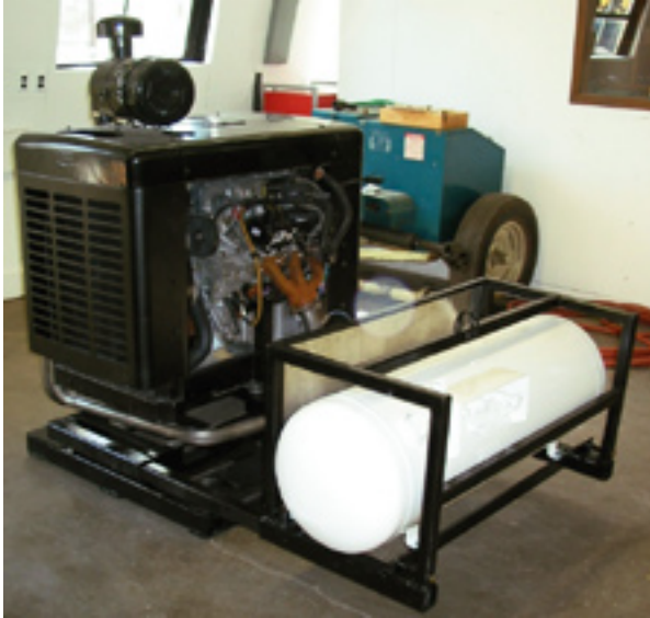
FIGURE 1. Ford ESG-642 propane engine equipped with DOT fuel tank. The M&W dynamometer is in the background.
