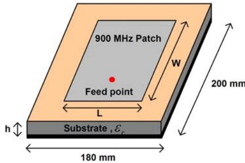
Fig. 3.4 Conventional microstrip patch antenna operating at 900 MHz
