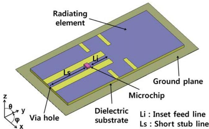
Fig. 4.7 Structure of the compact patch-type tag antenna
