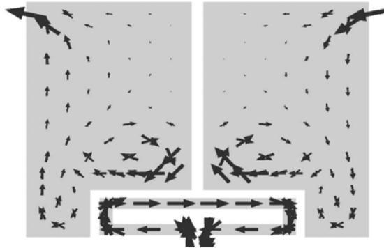
Fig. 4.3 Surface current distribution of balanced-type microstrip patches
