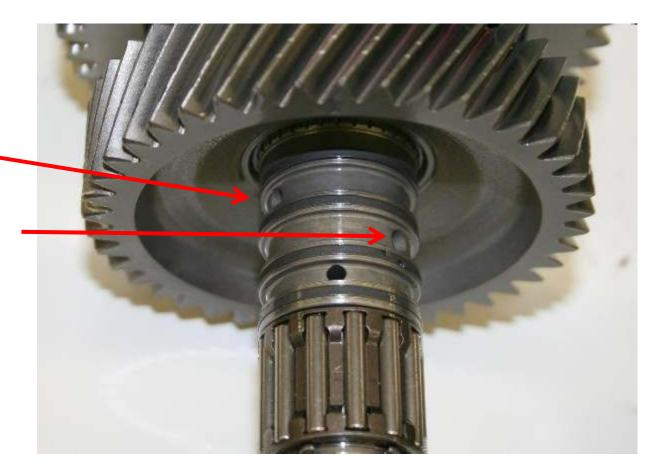
Check for arrows on the shaft nuts
