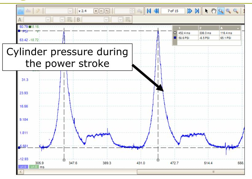
Exhaust valve opens. Initially the piston was going to return to a vacuum, since there is no combustion while performing a running compression test, but since the exhaust valve opened, pressure increased to exhaust system pressure
