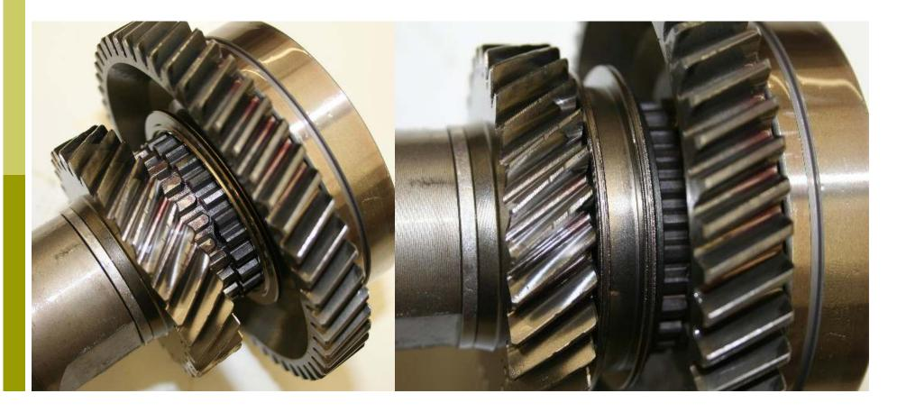
The outer race of the sprag should freewheel in the clockwise direction when positioned as shown
