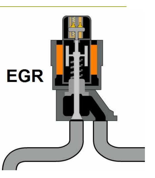
Look at when the EGR is commanded. At idle, there is no EGR; at cruise, EGR is modulated ON; at higher throttle position, EGR is removed. The PCM is calibrated to know approximately how much EGR is entering the cylinder and how much injector pulse width is needed to achieve proper A/F control. The O2 sensor then fine tunes the system.
