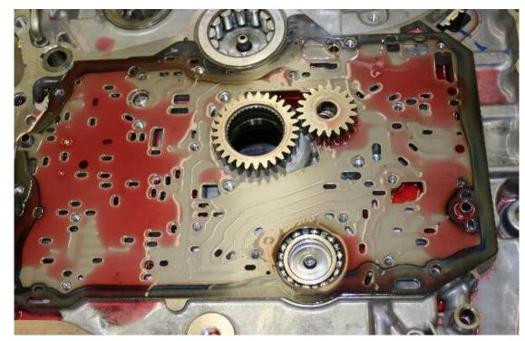
4th Gear is pressed onto the mainshaft with the bearing installed. You will damage the bearing if you remove this gear.
