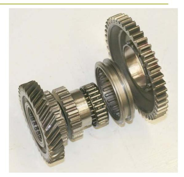
The 5<sup>th</sup> gear on the mainshaft has a lip/ledge on the bearing that must seat in the pocket in the gear
